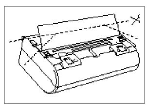
(8) Check the position of the top edge of film. It should be aligned with the cutting line of the cartridge. If any film extends beyond the cutting line, cut away the access film as illustrated before installing the cartridge.
